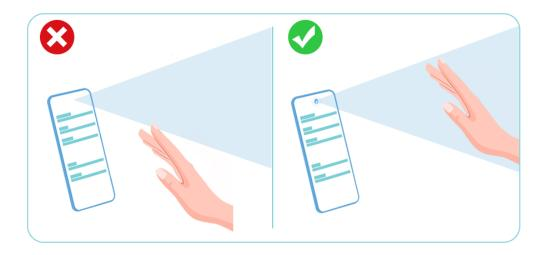
$\bf 3$  To scroll up, hold the back of your hand towards the screen with your fingers pointing down, then wave up when  $\stackrel{\frown}{\omega}$  appears.
